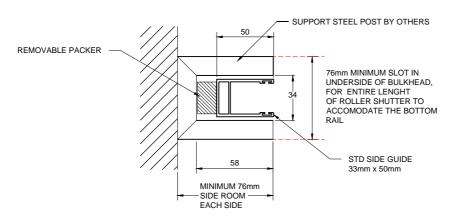
$\overline{\text{IMPORTANT}}$  WHEN USING THIS DETAIL, THE BULKHEAD MUST BE SUFFICIENTLY STRUCTURAL TO SUPPORT THE WEIGHT OF THE MOTORISED DOOR
